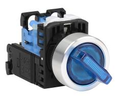
Fuji Electric selector switch, 22mm, 2-position, maintained, LED illuminated, (1) N.O. contact(s), plastic base, metal bezel, Operator: blue, knob, 30mm, round, plastic, 115-127 VAC, transformer.
