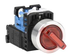
Fuji Electric selector switch, 22mm, 2-position, maintained, LED illuminated, (1) N.O. contact(s), plastic base, metal bezel, Operator: red, knob, 30mm, round, plastic, 115-127 VAC, transformer.
