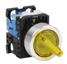
Fuji Electric selector switch, 22mm, 2-position, maintained, LED illuminated, (1) N.O. contact(s), plastic base, metal bezel, Operator: yellow, knob, 30mm, round, plastic, 24 VAC/VDC, full voltage.
