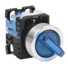
Fuji Electric selector switch, 22mm, 2-position, maintained, LED illuminated, (1) N.O. contact(s), plastic base, metal bezel, Operator: blue, knob, 30mm, round, plastic, 24 VAC/VDC, full voltage.
