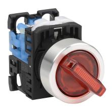
Fuji Electric selector switch, 22mm, 2-position, maintained, LED illuminated, (1) N.O. contact(s), plastic base, metal bezel, Operator: red, knob, 30mm, round, plastic, 24 VAC/VDC, full voltage.
