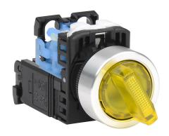
Fuji Electric selector switch, 22mm, 2-position, spring return from right, LED illuminated, (1) N.O. contact(s), plastic base, metal bezel, Operator: yellow, knob, 30mm, round, plastic, 115-127 VAC, transformer.
