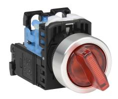
Fuji Electric selector switch, 22mm, 2-position, spring return from right, LED illuminated, (1) N.O. contact(s), plastic base, metal bezel, Operator: red, knob, 30mm, round, plastic, 115-127 VAC, transformer.
