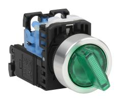
Fuji Electric selector switch, 22mm, 2-position, spring return from right, LED illuminated, (1) N.O. contact(s), plastic base, metal bezel, Operator: green, knob, 30mm, round, plastic, 115-127 VAC, transformer.
