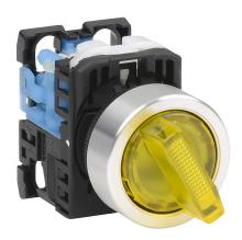
Fuji Electric selector switch, 22mm, 2-position, spring return from right, LED illuminated, (1) N.O. contact(s), plastic base, metal bezel, Operator: yellow, knob, 30mm, round, plastic, 24 VAC/VDC, full voltage.
