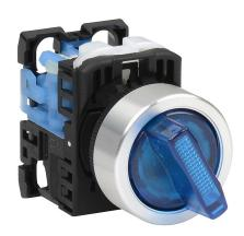
Fuji Electric selector switch, 22mm, 2-position, spring return from right, LED illuminated, (1) N.O. contact(s), plastic base, metal bezel, Operator: blue, knob, 30mm, round, plastic, 24 VAC/VDC, full voltage.
