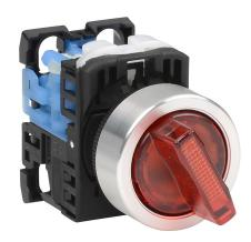
Fuji Electric selector switch, 22mm, 2-position, spring return from right, LED illuminated, (1) N.O. contact(s), plastic base, metal bezel, Operator: red, knob, 30mm, round, plastic, 24 VAC/VDC, full voltage.
