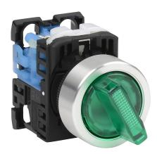
Fuji Electric selector switch, 22mm, 2-position, spring return from right, LED illuminated, (1) N.O. contact(s), plastic base, metal bezel, Operator: green, knob, 30mm, round, plastic, 24 VAC/VDC, full voltage.
