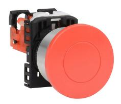
Fuji Electric pushbutton, 22mm, momentary, (1) N.C. contact(s), plastic base, metal bezel, Operator: red, mushroom, 40mm, round, plastic.
