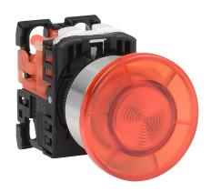
Fuji Electric pushbutton, 22mm, momentary, LED illuminated, (1) N.C. contact(s), plastic base, metal bezel, Operator: red, mushroom, 40mm, round, plastic, 24 VAC/VDC, full voltage.
