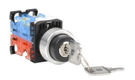
Fuji Electric selector switch, 22mm, 3-position, maintained, key removable left, right and center position, (2) N.O./(2) N.C. contact(s), plastic base, metal bezel, Operator: black, key, 30mm, round, plastic.
