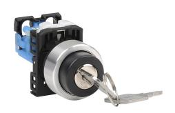
Fuji Electric selector switch, 22mm, 2-position, maintained, key removable left and right position, (1) N.O. contact(s), plastic base, metal bezel, Operator: black, key, 30mm, round, plastic.
