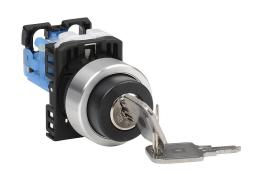
Fuji Electric selector switch, 22mm, 2-position, spring return from right, key removable left position, (1) N.O. contact(s), plastic base, metal bezel, Operator: black, key, 30mm, round, plastic.
