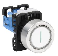
Fuji Electric pushbutton, 22mm, momentary, (1) N.O. contact(s), plastic base, metal bezel, Operator: white, flush, 30mm, round, plastic, operator text "(I)".
