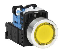
Fuji Electric pushbutton, 22mm, push ON - push OFF, LED illuminated, (1) N.O. contact(s), plastic base, metal bezel, Operator: yellow, flush, 30mm, round, plastic, 115-127 VAC, transformer.
