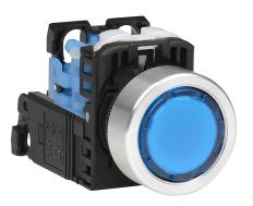
Fuji Electric pushbutton, 22mm, push ON - push OFF, LED illuminated, (1) N.O. contact(s), plastic base, metal bezel, Operator: blue, flush, 30mm, round, plastic, 115-127 VAC, transformer.
