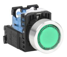
Fuji Electric pushbutton, 22mm, push ON - push OFF, LED illuminated, (1) N.O. contact(s), plastic base, metal bezel, Operator: green, flush, 30mm, round, plastic, 115-127 VAC, transformer.
