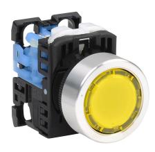
Fuji Electric pushbutton, 22mm, push ON - push OFF, LED illuminated, (1) N.O. contact(s), plastic base, metal bezel, Operator: yellow, flush, 30mm, round, plastic, 24 VAC/VDC, full voltage.
