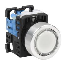
Fuji Electric pushbutton, 22mm, push ON - push OFF, LED illuminated, (1) N.O. contact(s), plastic base, metal bezel, Operator: white, flush, 30mm, round, plastic, 24 VAC/VDC, full voltage.
