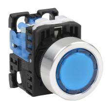
Fuji Electric pushbutton, 22mm, push ON - push OFF, LED illuminated, (1) N.O. contact(s), plastic base, metal bezel, Operator: blue, flush, 30mm, round, plastic, 24 VAC/VDC, full voltage.
