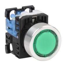
Fuji Electric pushbutton, 22mm, push ON - push OFF, LED illuminated, (1) N.O. contact(s), plastic base, metal bezel, Operator: green, flush, 30mm, round, plastic, 24 VAC/VDC, full voltage.
