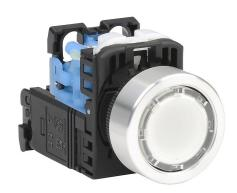
Fuji Electric pushbutton, 22mm, momentary, LED illuminated, (1) N.O. contact(s), plastic base, metal bezel, Operator: white, flush, 30mm, round, plastic, 115-127 VAC, transformer.
