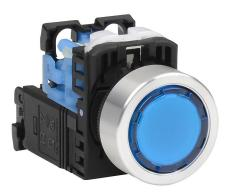
Fuji Electric pushbutton, 22mm, momentary, LED illuminated, (1) N.O. contact(s), plastic base, metal bezel, Operator: blue, flush, 30mm, round, plastic, 115-127 VAC, transformer.
