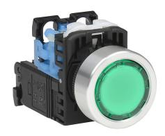
Fuji Electric pushbutton, 22mm, momentary, LED illuminated, (1) N.O. contact(s), plastic base, metal bezel, Operator: green, flush, 30mm, round, plastic, 115-127 VAC, transformer.
