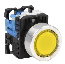
Fuji Electric pushbutton, 22mm, momentary, LED illuminated, (1) N.O. contact(s), plastic base, metal bezel, Operator: yellow, flush, 30mm, round, plastic, 24 VAC/VDC, full voltage.
