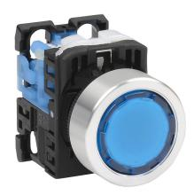
Fuji Electric pushbutton, 22mm, momentary, LED illuminated, (1) N.O. contact(s), plastic base, metal bezel, Operator: blue, flush, 30mm, round, plastic, 24 VAC/VDC, full voltage.
