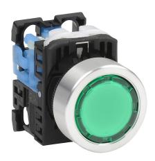
Fuji Electric pushbutton, 22mm, momentary, LED illuminated, (1) N.O. contact(s), plastic base, metal bezel, Operator: green, flush, 30mm, round, plastic, 24 VAC/VDC, full voltage.
