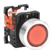
Fuji Electric pushbutton, 22mm, momentary, LED illuminated, (1) N.C. contact(s), plastic base, metal bezel, Operator: red, flush, 30mm, round, plastic, 24 VAC/VDC, full voltage.
