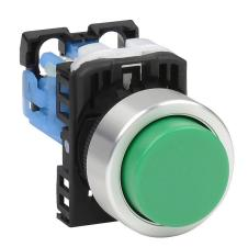
Fuji Electric pushbutton, 22mm, momentary, (1) N.O. contact(s), plastic base, metal bezel, Operator: green, extended, 30mm, round, plastic.
