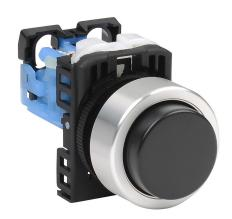
Fuji Electric pushbutton, 22mm, momentary, (1) N.O. contact(s), plastic base, metal bezel, Operator: black, extended, 30mm, round, plastic.
