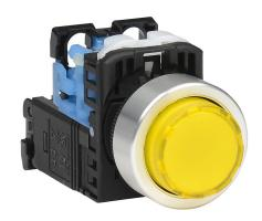
Fuji Electric pushbutton, 22mm, momentary, LED illuminated, (1) N.O. contact(s), plastic base, metal bezel, Operator: yellow, extended, 30mm, round, plastic, 115-127 VAC, transformer.
