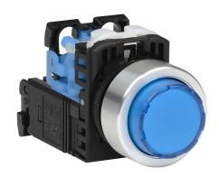
Fuji Electric pushbutton, 22mm, momentary, LED illuminated, (1) N.O. contact(s), plastic base, metal bezel, Operator: blue, extended, 30mm, round, plastic, 115-127 VAC, transformer.
