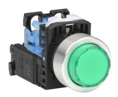
Fuji Electric pushbutton, 22mm, momentary, LED illuminated, (1) N.O. contact(s), plastic base, metal bezel, Operator: green, extended, 30mm, round, plastic, 115-127 VAC, transformer.
