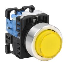
Fuji Electric pushbutton, 22mm, momentary, LED illuminated, (1) N.O. contact(s), plastic base, metal bezel, Operator: yellow, extended, 30mm, round, plastic, 24 VAC/VDC, full voltage.
