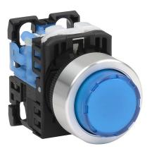
Fuji Electric pushbutton, 22mm, momentary, LED illuminated, (1) N.O. contact(s), plastic base, metal bezel, Operator: blue, extended, 30mm, round, plastic, 24 VAC/VDC, full voltage.
