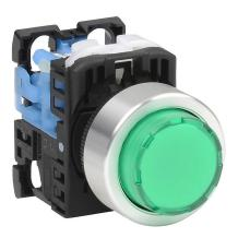
Fuji Electric pushbutton, 22mm, momentary, LED illuminated, (1) N.O. contact(s), plastic base, metal bezel, Operator: green, extended, 30mm, round, plastic, 24 VAC/VDC, full voltage.
