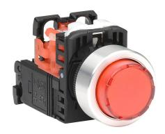
Fuji Electric pushbutton, 22mm, momentary, LED illuminated, (1) N.C. contact(s), plastic base, metal bezel, Operator: red, extended, 30mm, round, plastic, 115-127 VAC, transformer.
