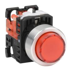
Fuji Electric pushbutton, 22mm, momentary, LED illuminated, (1) N.C. contact(s), plastic base, metal bezel, Operator: red, extended, 30mm, round, plastic, 24 VAC/VDC, full voltage.
