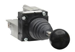
Fuji Electric selector switch, IP65, 22mm, 2-position, momentary, (2) N.O. contact(s), plastic base, plastic bezel, Operator: black, joystick, 30mm, round, plastic.
