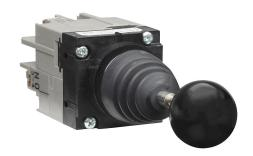
Fuji Electric selector switch, IP65, 22mm, 4-position, maintained, (4) N.O. contact(s), plastic base, plastic bezel, Operator: black, joystick, 30mm, round, plastic.
