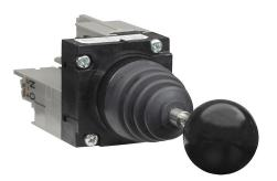
Fuji Electric selector switch, IP65, 22mm, 2-position, maintained, (2) N.O. contact(s), plastic base, plastic bezel, Operator: black, joystick, 30mm, round, plastic.
