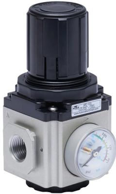
NITRA pneumatic regulator, 3/8in female NPT inlet(s), 3/8in female NPT outlet(s), 7-130 psi range. For use with Ax-33 series air prep components.
