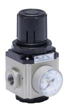
NITRA pneumatic regulator, 1/4in female NPT inlet(s), 1/4in female NPT outlet(s), 7-60 psi range. For use with Ax-22 series air prep components.
