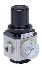
NITRA pneumatic regulator, 1/8in female NPT inlet(s), 1/8in female NPT outlet(s), 7-130 psi range. For use with Ax-21 series air prep components.
