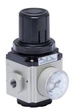
NITRA pneumatic regulator, 1/8in female NPT inlet(s), 1/8in female NPT outlet(s), 7-60 psi range. For use with Ax-21 series air prep components.
