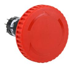
Fuji Electric emergency stop pushbutton, IP65, 16mm, push to lock, pull or turn to reset, (1) N.O./(3) N.C. contact(s), plastic base, plastic bezel, black, Operator: red, mushroom, 40mm, mushroom, plastic.
